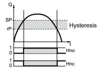
The hysteresis keeps the switch status of the output stable if the flow fluctuates around the nominal value.
