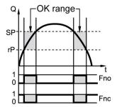
The window function allows a defined OK range to be monitored.
