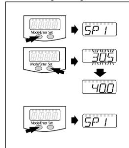
Press [Mode/Enter] until the desired parameter appears in the display.
